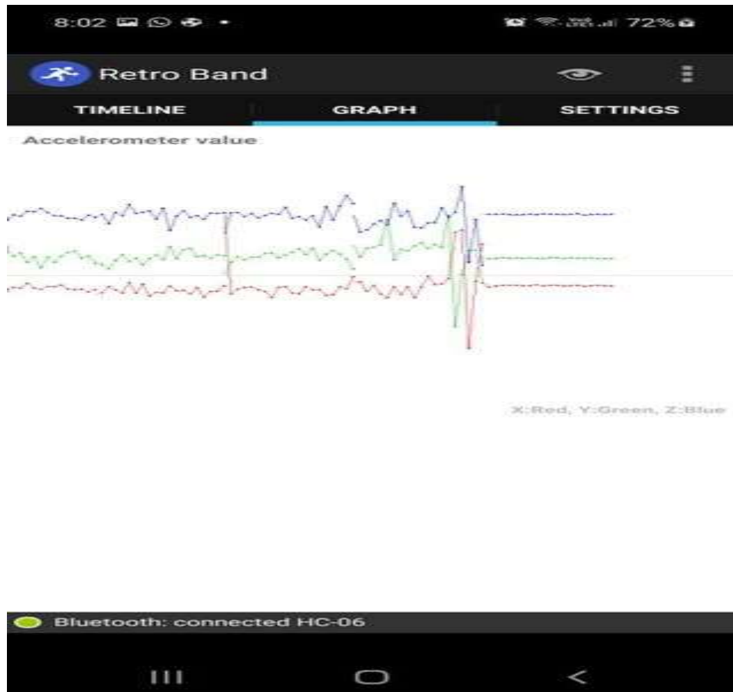
Figure 6. Accelerometer data successfully sent to app via BLE
