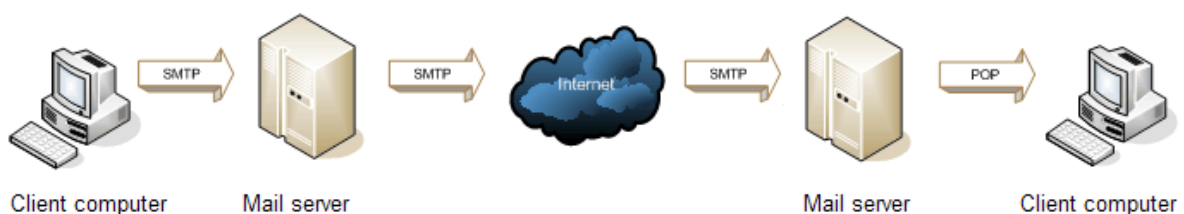
Figure 9: How an email server operates (What is a Mail Server and How Does it Work? (Article), 2020)
